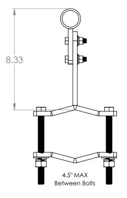
Will mount on tower legs from 1.5" to 4.5" dia. Reversing the outer clamp allows it to be attached to angle iron tower legs.
